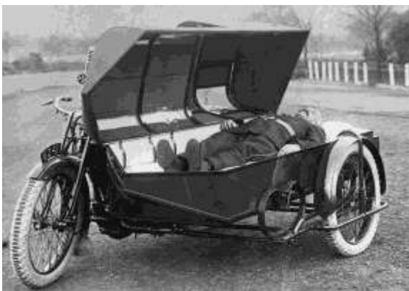
An early ambulance operated by St John. The patient was placed in a coffin-like sidecar and the lid was closed for transport. There was however a couple of hatches
